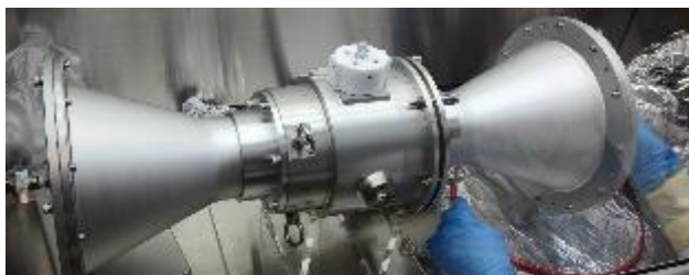
Fig. 8. Each component of the sampling unit was sterilized, then assembled and sealed inside a clean bench.
