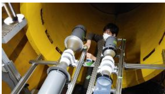
Fig. 7. Wind tunnel experiment to test the sampling unit using JAXA's Planetary Environment Wind Tunnel.
