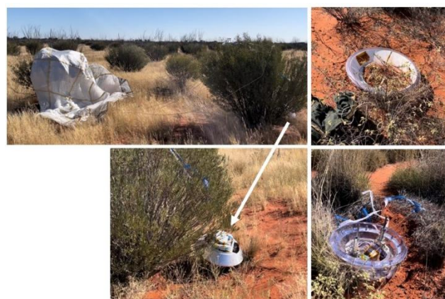
Fig. 7. Photos of the parachute (left upper), the instrument module (left lower), the back heat shield (right upper) and the front heat shield (right lower), at recovery.
