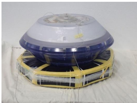
Fig. 3. Photo of the experimental SRC for the flight test
