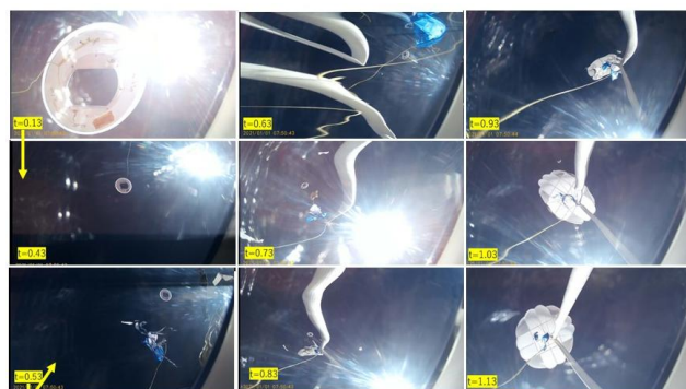
Fig. 15. Sequential images captured by the onboard camera during the parachute deployment at 0.1 second intervals.
